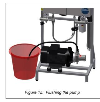
Remove plugs and strips from the highpressure hose and lead it to a drain or a bucket.
