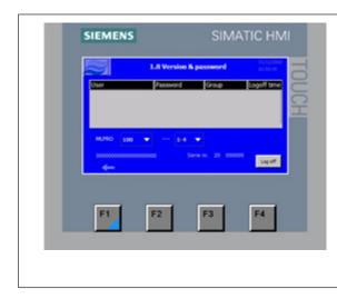
Select MLP size and select 1-4 or 1-8 sections. This selection is pre-set from factory according to the controller hardware.
