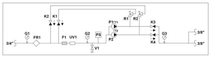
Figure 9: Hydraulic diagram MLP 2x800
