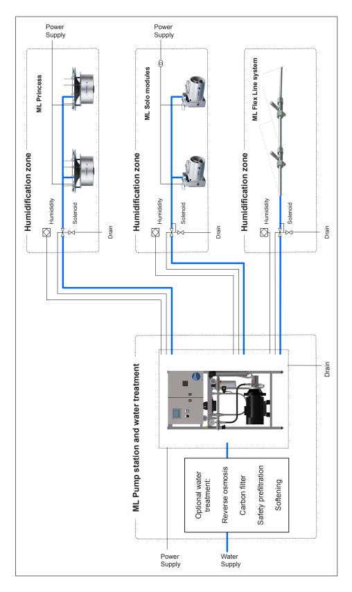
Figure 10: Principal installation diagram
