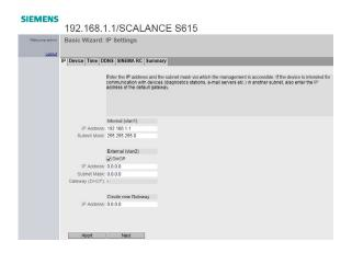
Enter under "Internal (vlan1)": IP Address: 192.168.100.200 Subnet Mask: 255.255.255.0
