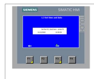
Time/date can be set (stored in the screen only). Note: Remember to press F3 to set the PLC clock
