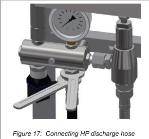
Turn S1 (on/off switch) to off position, and connect the HP discharge hose to the high-pressure manifold.
