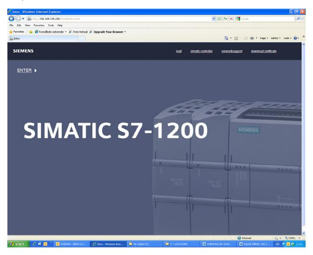
After entering the correct IP address - the following picture appears. Start by downloading and installing Siemens security certificate (download and follow the onscreen instructions). Then press Enter
